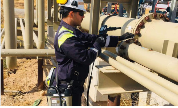
Dhabyan Zand from Intero - The Sniffers measuring fugitive emissions with an FID device (TVA2020)
