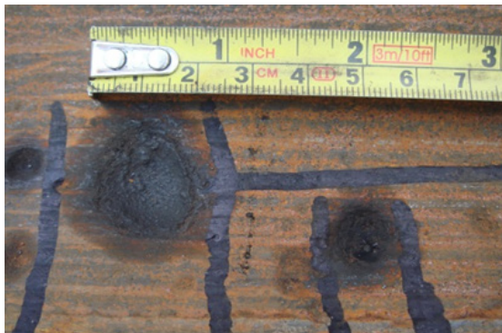
Actual picture of the tube with pitting corrosion.
