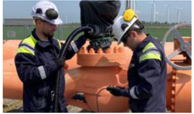
Quantifying methane losses with a High Flow Sampler (HFS).
